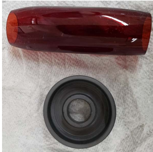
Figure 1. Image of Thermal Quartz (top) and Silicon Carbide Crucible (bottom)
